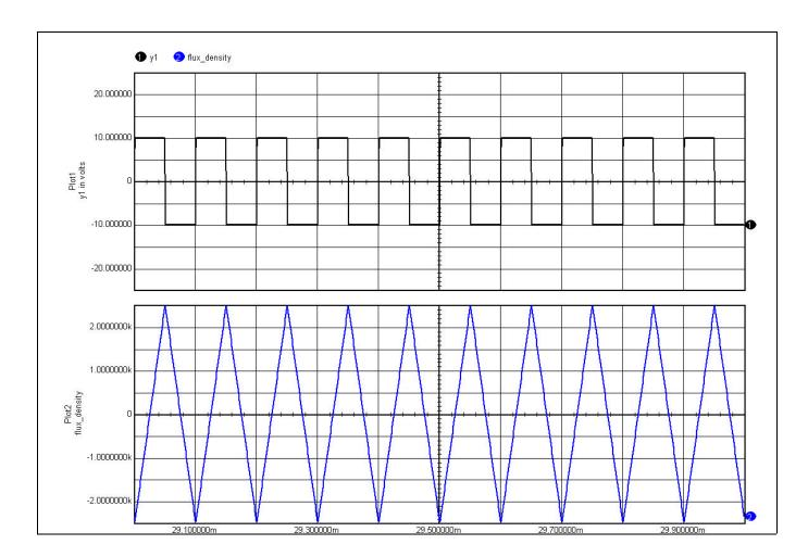
The top waveform is the applied voltage and the bottom waveform is the resulting core flux (in gauss) for a hypothetical core I have modeled. The following plot shows the B-H loop (vertical axis is B & horizontal axis is current which is proportional to H). We can see that, in this case, we have volt-second balance and the core does not walk.
