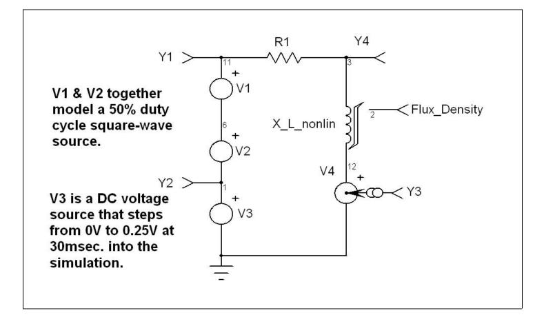
For simplicity, only the transformer primary winding is shown.
