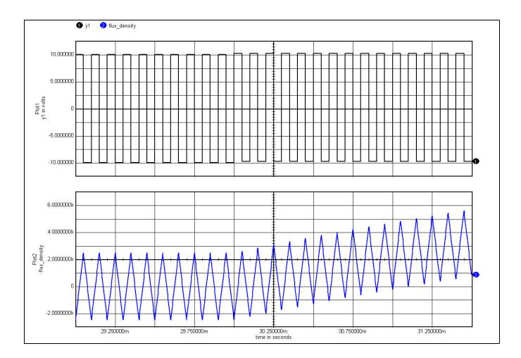
We can see that, in this case, we do not have volt-second balance and the core walks. The corresponding B-H loop will clearly illustrate flux-walking and the onset of core saturation:
