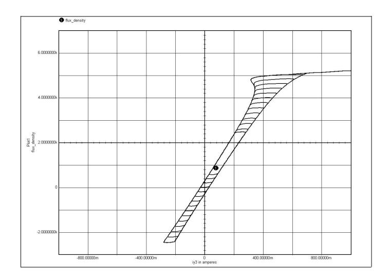
The transformer can clearly be seen walking to saturation. The result (without limiting) is an explosion in the converter power stage. Not good!!
